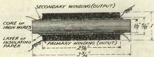
Fig. 1.—Section of completed transformer, showing dimensions.
